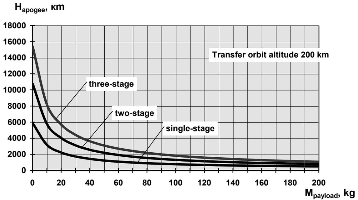
Some estimates of the orbit parameters provided by the two-stage TOR are given in the table below (the altitude of transfer orbit is 200 km).
