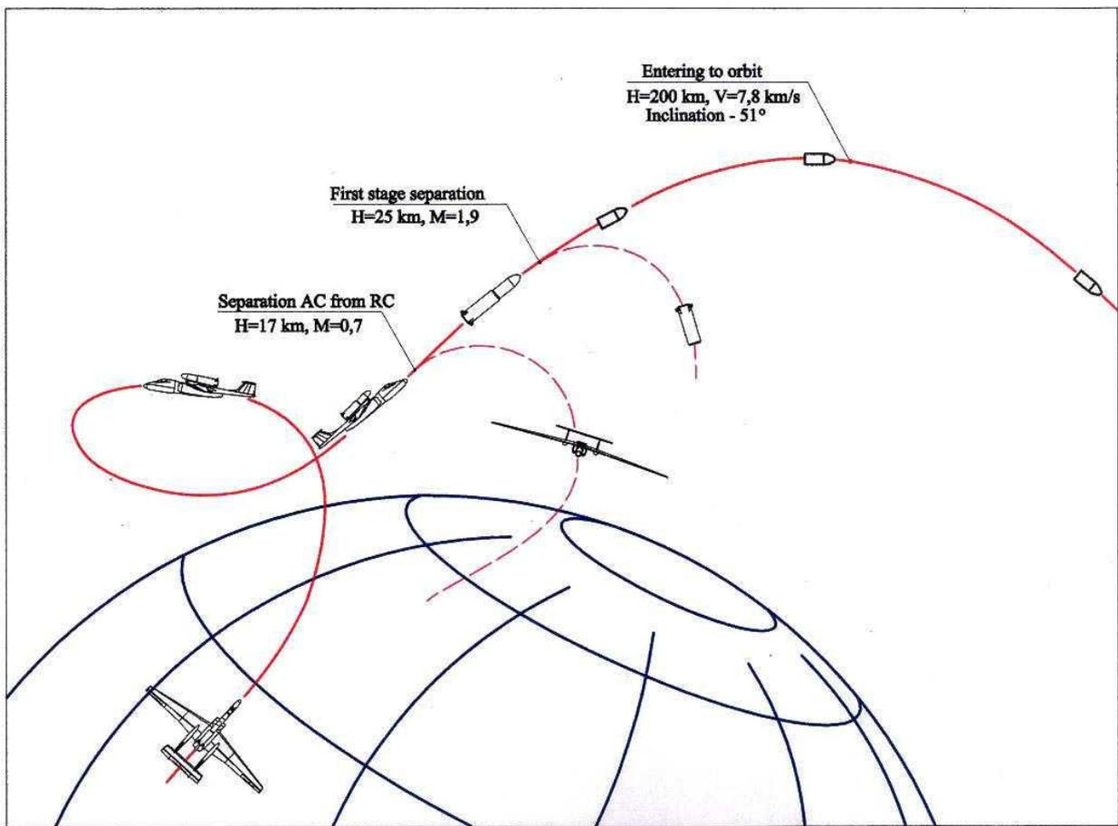
Calculations made for the rocket-carrier (RC) of 5500 kg mass, latitude of start  $47^\circ$  and inclination of orbit  $51^\circ$  have shown that the mass of payload (micro-satellite plus acceleration block), which can be inserted onto 200 km circular orbit, ranges from 100 to 150 kg depending on the RC parameters.
