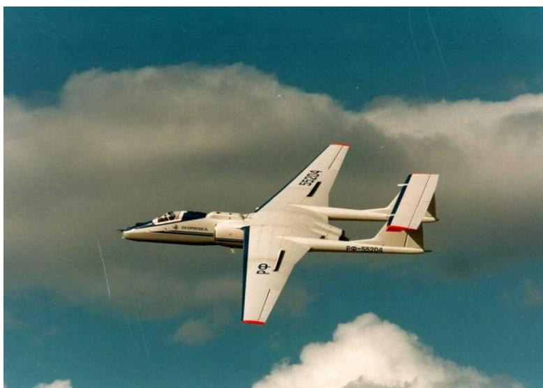
M-55 high altitude subsonic aircraft is an all metal twin-boom high-wing monoplane of normal configuration with a straight high-aspect ratio wing, a twin-finned tail unit, tricycle nose-
